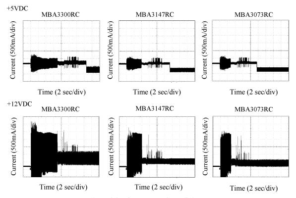
Figure 4.6 Current waveform (Spin-up)
